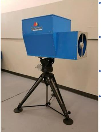
•A light source is transmitted down a clear path, often hundreds of meters, to measure what is in the air
