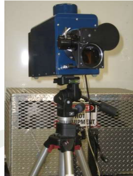
SOC750 Hyper- spectral imager 42 spectral channels, operated at 22 cubes per sec.
