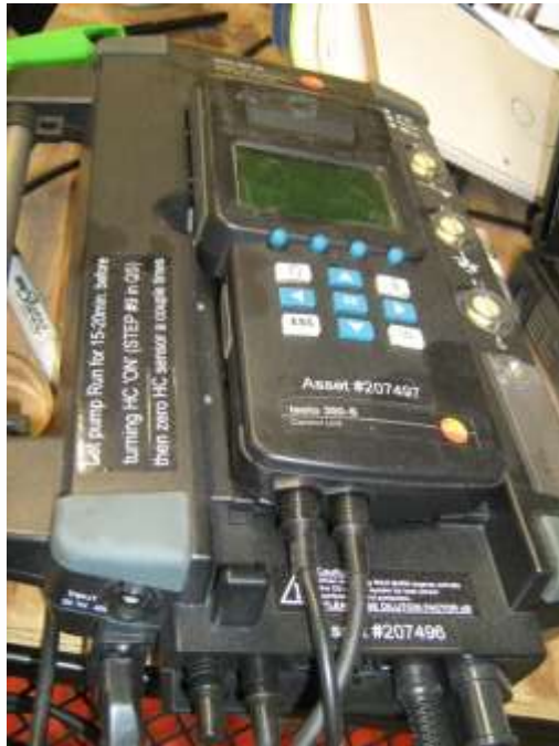
Testo 350 XL (CO 2 using NDIR, CO, O 2 , NO x , H 2 , Temp, etc.)
