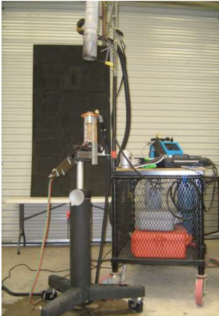
Scale model flare, Flue w/ Sampling Probe, and Analyzers
