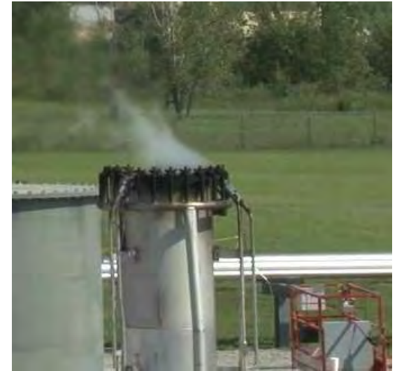
As the SVG almost doubles again to 1.05, the flare DRE drops to 27%. Note the flame has disappeared.
