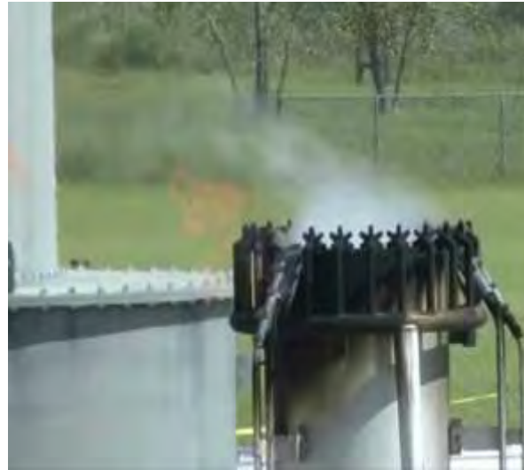
As the SVG almost doubles to 0.54, the flare DRE decreases to 90.6%. Note the flame is disappearing.
